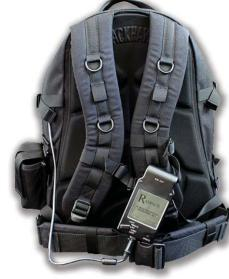
RadPack Max. RadPack Max is the most sensitive man-wearable neutron and gamma detector available. It employs an array of seven two-inch diameter Helium-3 tubes as neutron detectors, as well as six individual 1×4"cesium iodide gamma scintillators for gamma radiation sensing. Developed specifically for military operators, law enforcement, and first responders, the RadPack Max is lightweight, compact, and enjoys a level of ruggedness not approached by competing equipment.
